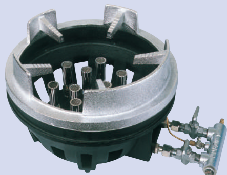
8-6 9本立 ■LPG/27,900Kcal/H, 32.4Kw/H, 2.33kg/H ■12, 13A/27,000Kcal/H, 31.3Kw/H, 2.45m 3 /H
